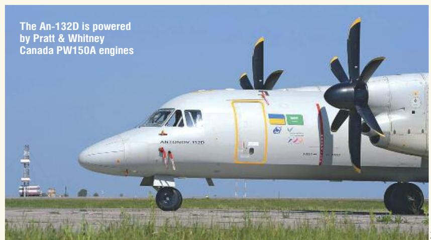
The An-132D is powered by Pratt & Whitney Canada PW150A engines
