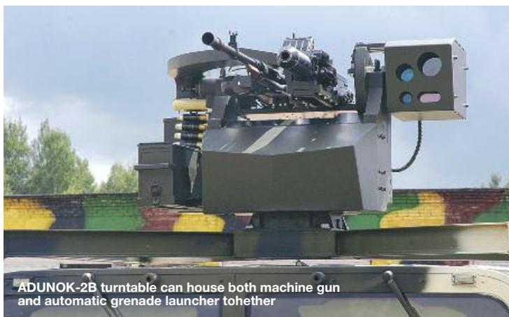
ADUNOK-2B turntable can house both machine gun and automatic grenade launcher together
