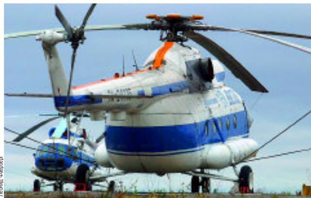
Equipping a Mil Mi-8MT with the new Motor-Sich TV3-117VMA-SBM1V turboshaft would increase the helicopter's external load capacity up to 6 tons
