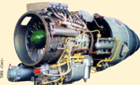
The 1,700-kgf-thrust RD-1700 has been developed to replace French Larzac at the Russian MiG-AT advanced jet trainer
