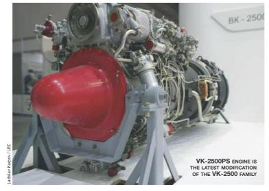
Mi-172s with only minimal modifications required for each rotorcraft. Other positives are that the timeframe before the required overhaul of the VK-2500PS-03 has increased and the assigned life is expected to increase to 12,000 hours.
