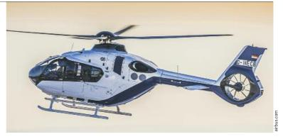
With a maximum take-off weight of 2,980 kilos, the helicopter is capable of carrying up to 1,417 kilos of payload inside the cabin, or 1,200 as an external load. The transport version of the helicopter is able carry up to seven passengers, while the medevac version can manage one to two patients with two to four attendants. The rotorcraft has a top speed of 259 km/h
