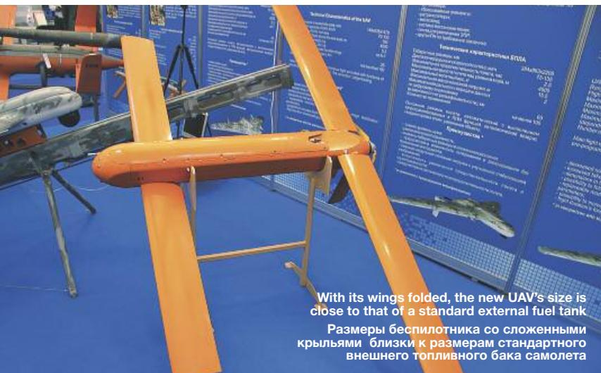
With its wings folded, the new UAV's size is close to that of a standard external fuel tank
